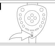
Slide the MIC/OFF/ON switch to the OFF position to turn the microphone off.
